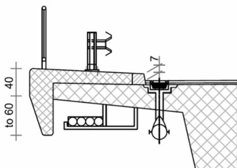
Fig. 5.1: Edge beam with raised vertical end up to 1.0 m
