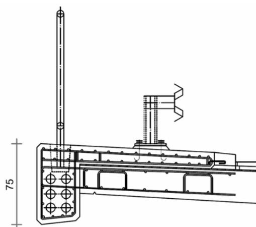
Fig. 5.1b: 6 ducts of  $\varnothing 80$  mm in the edge beam
