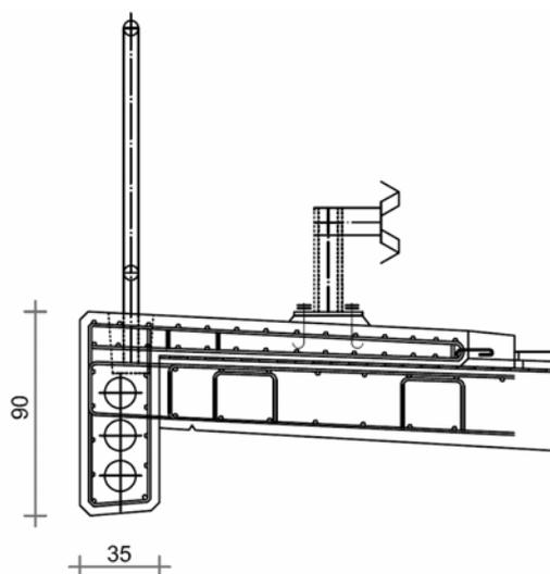
Fig. 5.1a: 3 ducts of  $\varnothing 125$  mm in the edge beam
