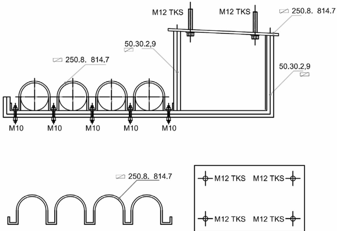
Fig. 9.2: Workshop drawing of suspension for four ducts
