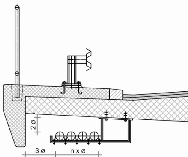
Fig. 9.1: Detail of fastening of installations below cantilever
